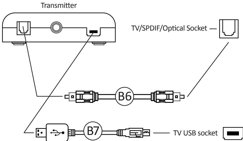
1. Connect **B6** Optical Cable to the **B3** Wirelessss DAC transmitter's SPDIF Port.
