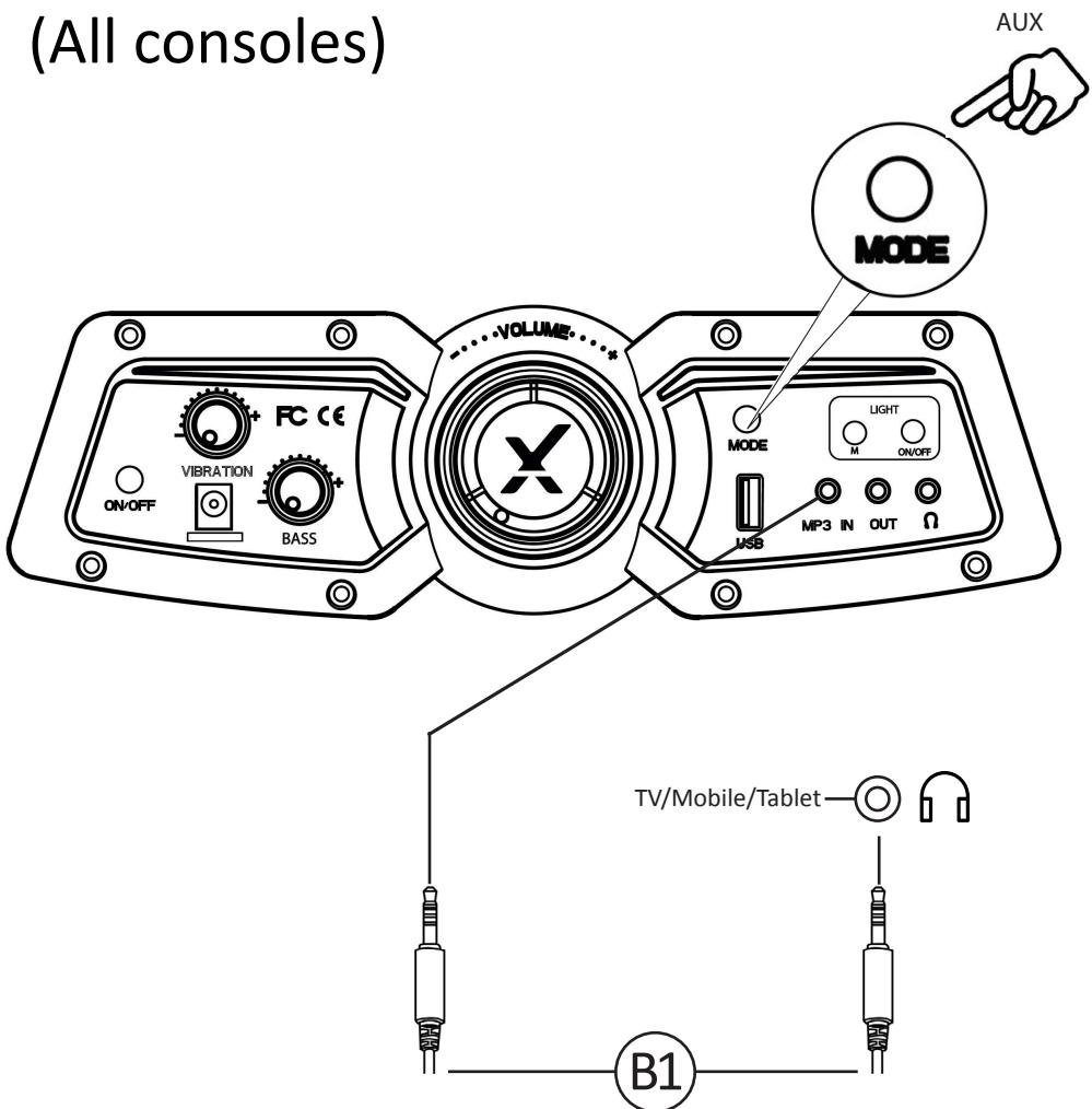
1. Connect **B1** Cable to X Rocker control panel MP3 INPUT sockets.
