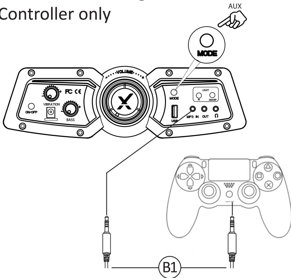
1. Connect the **B1** cable to the bottom of the PS4 controller via the headset socket.
